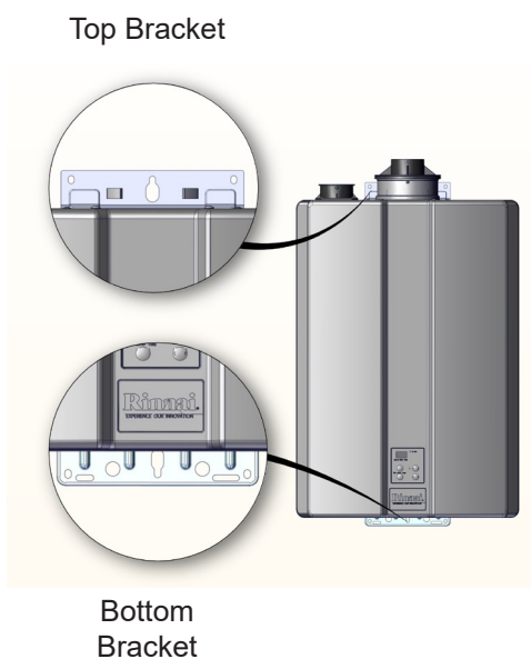
Figure 12: Mount the bottom bracket
